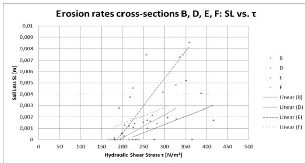
**Fig. 16:** Erosion rates in cross-sections B, D, E, F; regarding soil loss and shear stress, the steeper the trend line the higher the erosion rate
