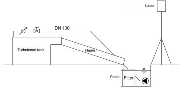
**Fig. 4:** Basic experimental set-up with laser scanner (Lesch 2012)
