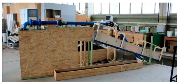
Fig. 1: Laboratory flume, sample boxes in the front, Chair of Geotechnics and Coastal Engineering
