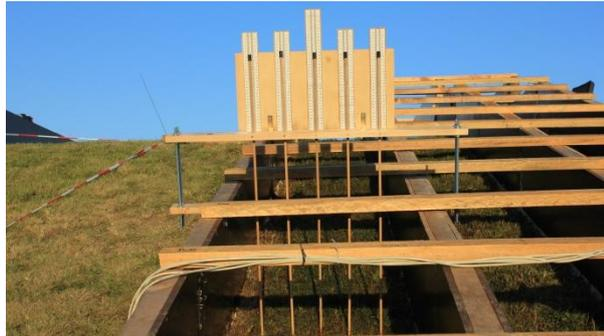
**Fig. 12:** Pin profiler to measure the soil loss/ gain and the discharge depth
