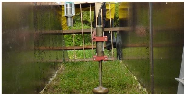
**Fig. 13:** Ultrasonic sensor to measure runoff depth (left), magnetic-inductive sensor to measure flow velocity (right)
