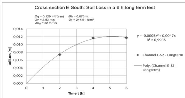
**Fig. 17:** Soil loss on cross-section E - long-term test
