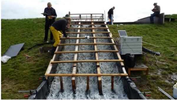
**Fig. 9:** Basic experimental set-up and procedure, cross-section H, first discharge stage ( $q \approx 50 \text{ ls}^{-1}\text{m}^{-1}$ ,  $v \approx 1.57 \text{ ms}^{-1}$ ,  $\tau \approx 270 \text{ Pa}$ ), measurement of flow velocity in the left flume, 6<sup>th</sup> test section
