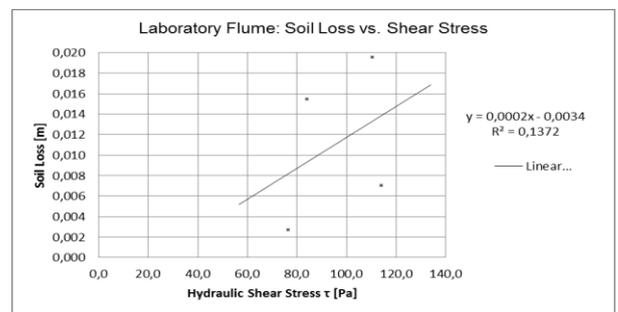
**Fig. 8:** Cumulated soil loss versus shear stress, only significant case of erosion in the course of laboratory flume tests with vegetated samples (M2, December 2013)
