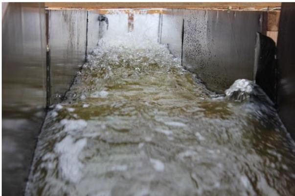
Fig. 18. Turbulent water surface, a lot of air entrainment in the lower area of the slope resp. flume
