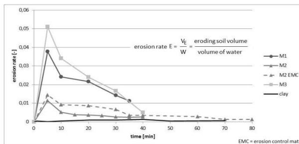
**Fig. 6:** Erosion rates of dredged materials (M1-M3) and clay (Cantré et al. 2013)
