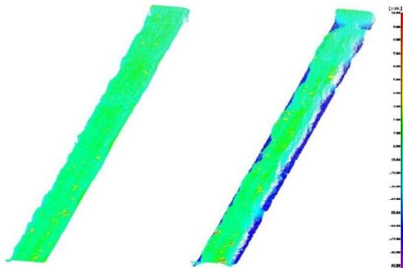
**Fig. 5:** Laser scan after overflowing events on material M3, after 5 minutes (left), after 15 minutes (right), dark blue = -70 mm soil loss, green = +/-0 mm soil loss/gain, red = +10 mm soil gain,  $\phi$  soil loss  $\approx 18,5$  mm ( $q \approx 3,2$   $ls^{-1}m^{-1}$ ,  $v \approx 0,22$   $ms^{-1}$ ,  $\tau \approx 10$  Pa)[JO2]
