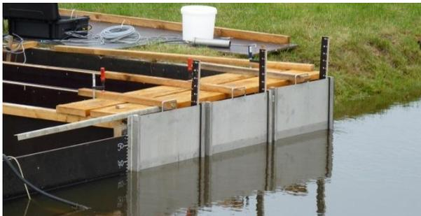
**Fig. 10:** Closed sluice gates at cross-section H
