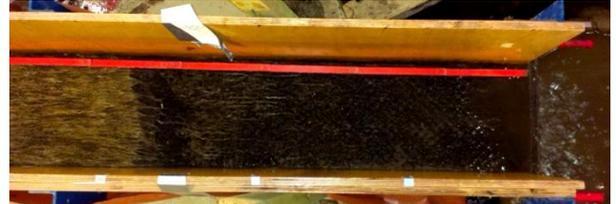
**Fig. 7:** Downstream erosion above the geomat (GMA), originate at a crosswise crack (M2, December 2013)
