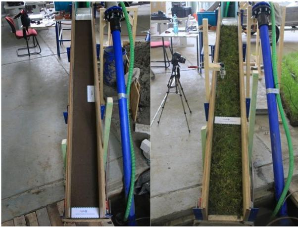
**Fig. 3:** Installed soil samples, unvegetated (left) and vegetated (right)
